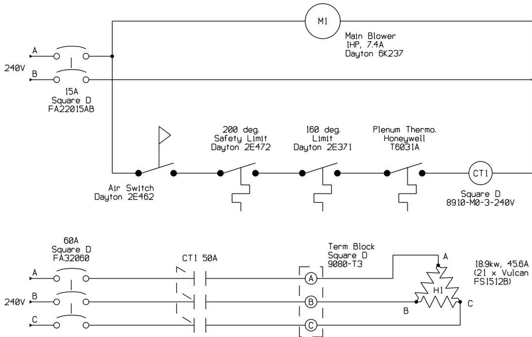
Figure 6: Ceiling Heat Circuit
