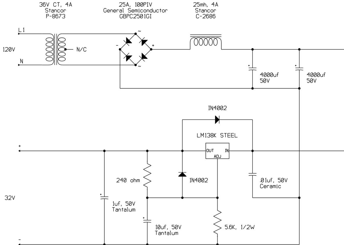
Figure 8: 32V, 4A DC Power Supply
