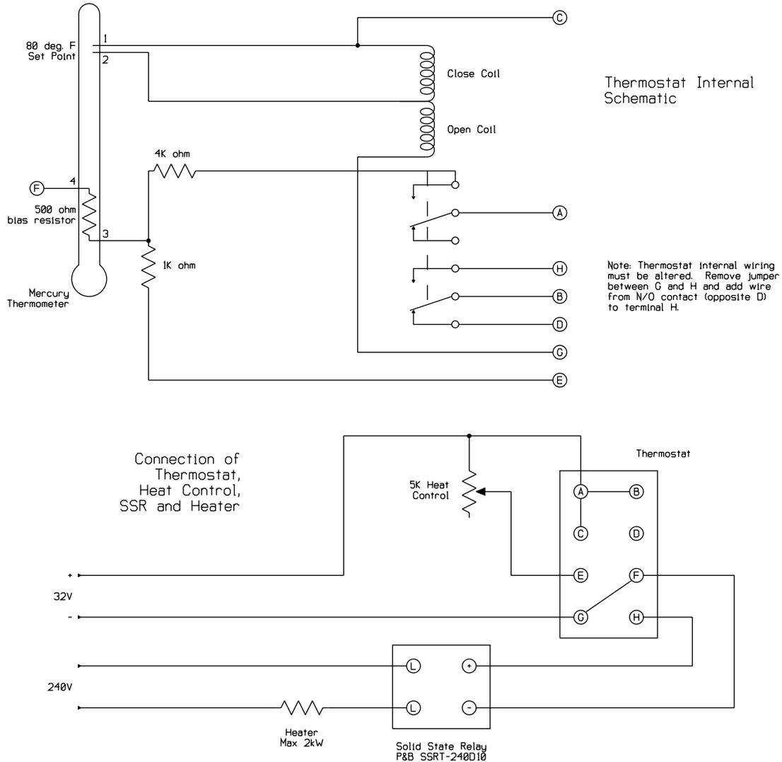
Figure 7: Using a Vapor Thermostat for Modern Heat Control
