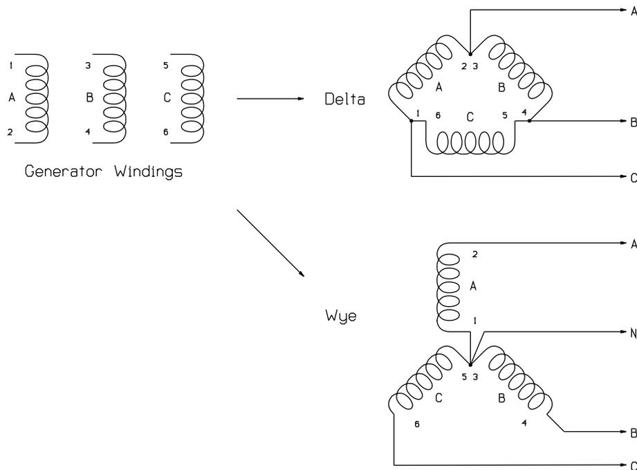
Figure 2: Connecting Windings as Delta or Wye
