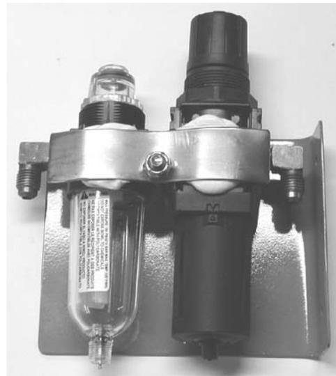
Photo 2 – A mini-FRL mounted on a bracket with a metal clip and copious glob of silicone caulking.
