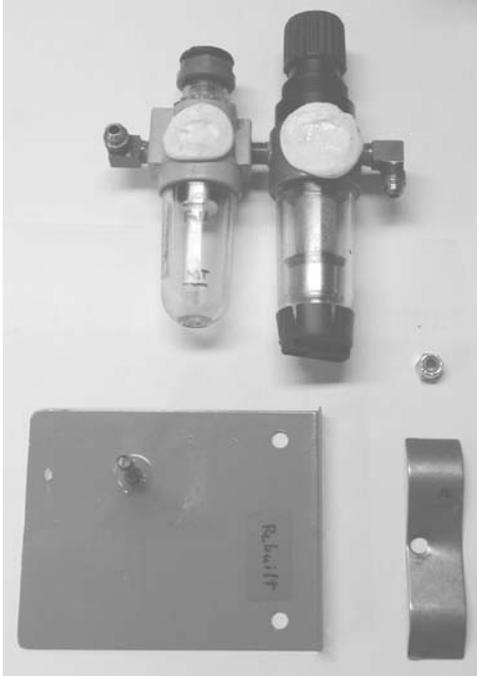
Photo 3 – FRL bracket, disassembled.
