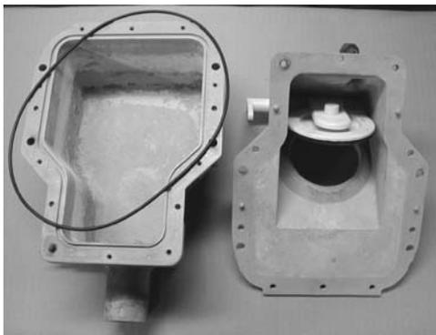
Photo 18 – Ejection chamber, disassembled, showing o-ring and flapper valve.
