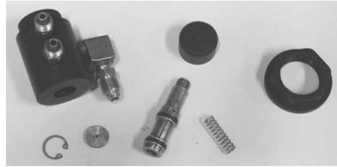
Photo 17 – Pushbutton valve disassembled for rebuilding.
