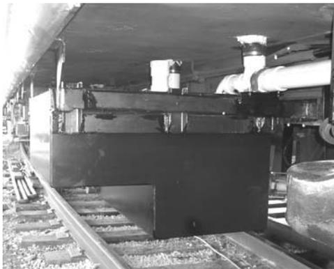
Photo 15 – All the connections to the Birch Grove's holding tank enter via the top. Disconnecting them would allow the tank to drop down and be easily removed. *Photo, September 2003, Sea Island Passenger Co.*
