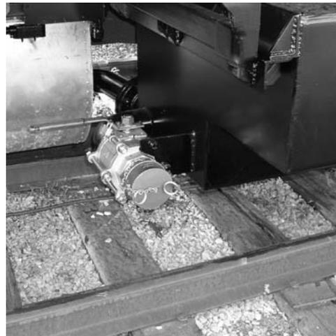
Photo 14 – The new holding tank on the Birch Grove has a conveniently located pumpout fitting. *Photo, September 2003, Sea Island Passenger Co.*
