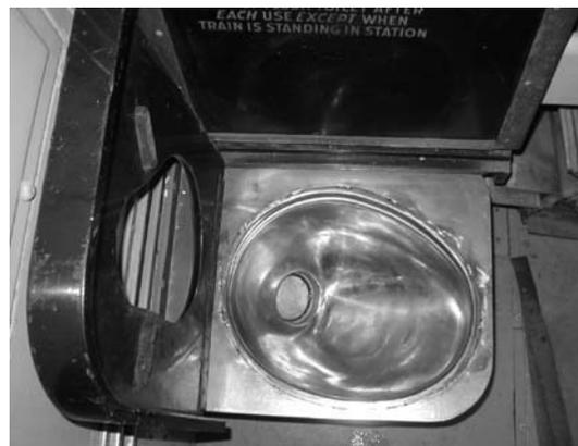
Photo 12 – The finished toilet. Installed in a roomette with the seat applied on top.
