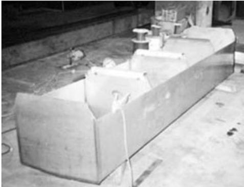
Photo 13 – A holding tank being fabricated for the Coffee Creek clearly shows the use of baffles to prevent sloshing. *Photo in April of 2003 by Taylor Johnson (www.coffeecreek.info).*
