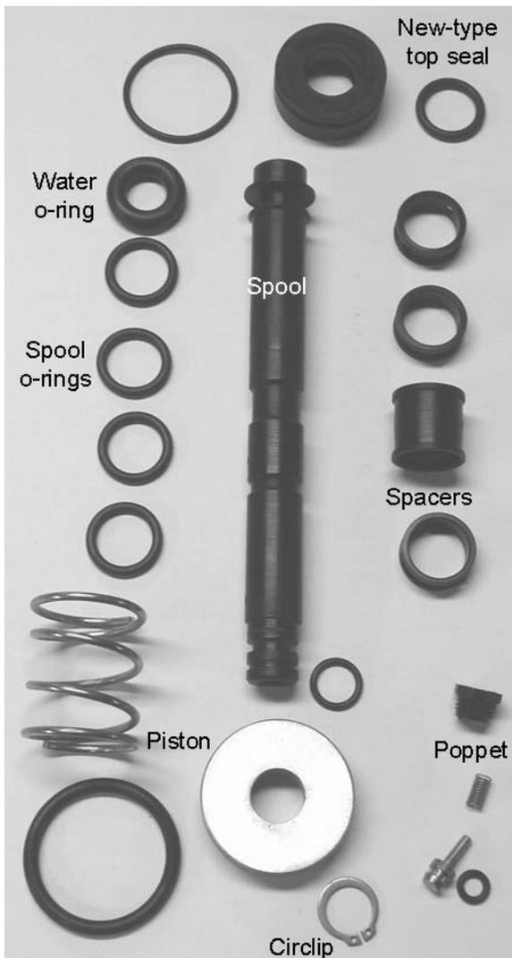
Photo 16 – AWS valve parts, more or less in order from top to bottom.
