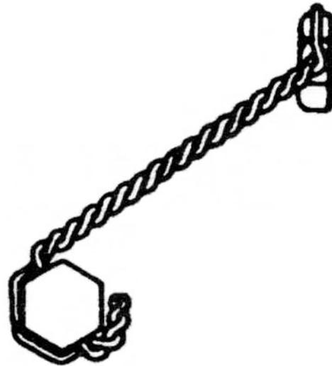
Figure 6: Wiring perpendicular fasteners.
