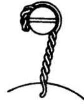
Figure 5: Wiring a fastener to a fixed object.
